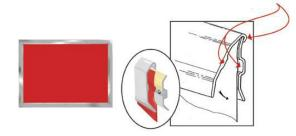
Apply direct pressure to Cover Plate while inserting screws, provided by Ackland. Vinyl will stretch, as screws are tightened. KEEP DRILL ON FAIRLY LOW SETTING to avoid OVERTIGHTENING/stripping. When screws are tight, and vinyl is wrinkle-free "tight as a drum"... CONGRATULATIONS!
